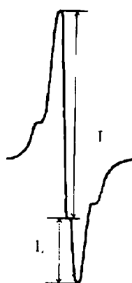
Fig. 3. ESR spectrum of cellulose irradiated at 300 K: I_1 ) intensity of the line sensitive to the crystal structure of cellulose; I_2 ) intensity of the line sensitive to the amorphous structure of cellulose.
